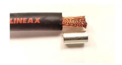
5. Fit the correct end sleeve or combination of end sleeves (see table below) over the conductor strands. Take care to ensure all the wire strands are inside the end sleeve
