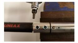
7. Now insert the contact into the rear of the insulator and align the hole in the contact so that it is in line with the holes in the insulator.
