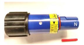
8. Now align the dowel pin with the tapered end first with the hole in the insulator. The dowel pin is designed to be a <u>tight interference fit</u> with insulator hole and it is necessary to drive the pin using a hammer through the insulator and contact. When fully inserted the pin will be flush with the surface of the insulator body.
