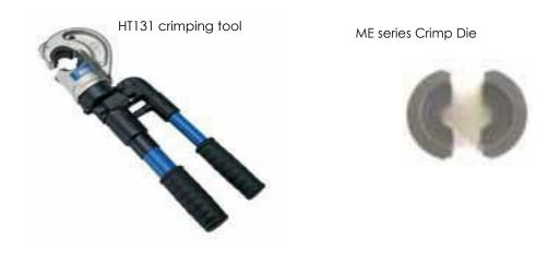
1. A hydraulic crimping tool and hexagonal Die set is used to perform a crimp termination. Selection of the correct crimp die is essential to achieve a reliable result. As cable conductor sections vary widely, the table below is intended as a guide to appropriate die selection. Cable tensile test should be performed to ensure the final crimp termination meets the tensile and my drop test of a particular specification.
