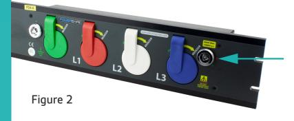
**5.** When the L3 connector is mated and turned fully clockwise to the locked position, take the key lock and turn the L3 lock clockwise. (Fig 2).
