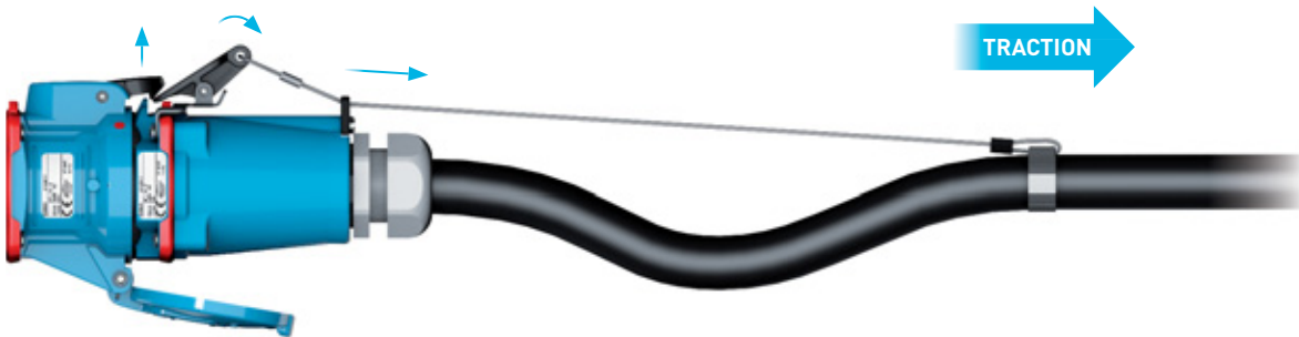
Step 2: the traction acts on the electrical cable and the rope. The ejection finger gradually raises the latch.
