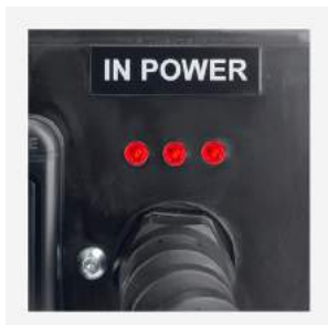
Red lights signal input voltage presence
