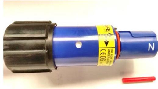
8. Now align the dowel pin with the tapered end first with the hole in the insulator. The dowel pin is designed to be a tight interference fit with insulator hole and it is necessary to drive the pin using a hammer through the insulator and contact. When fully inserted the pin will be flush with the surface of the insulator body.
