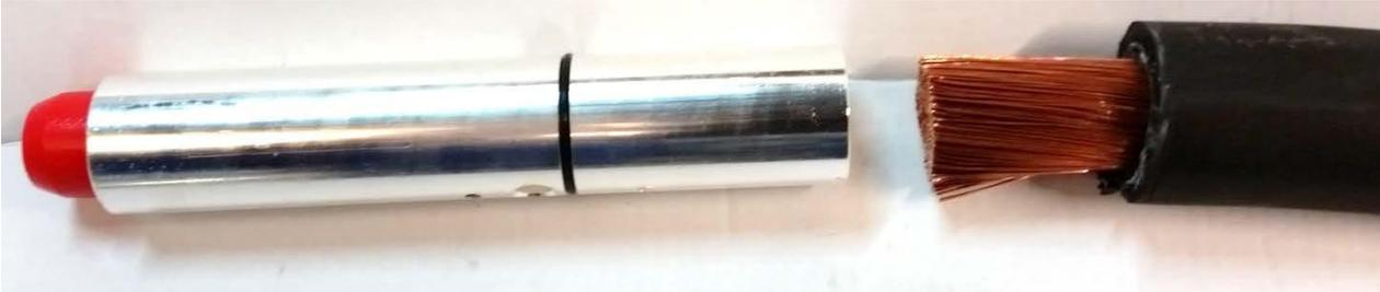
3: Slide the conductor into the rear of the contact. Take care to ensure all the wire strands are inside the contact.
