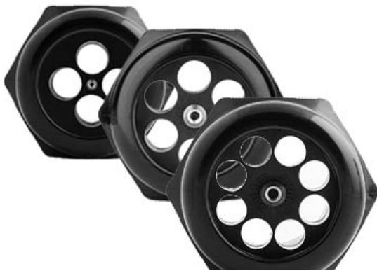
SYNTAX® SSX SPIDER connectors are alternative versions of standard 19-pin SSX flying connectors, designed for quick and easy management of breakout applications. The Syntax patented 4, 6 or 8-way rubber cable glands, mounted in the cable gland, ensure optimal cable tightness and an IP67 watertight seal for outdoor use. For assembly with 6 cables, the use of the Syntax® MAINFLEX cable is recommended for complete IP67 waterproof protection and the best maneuverability.
