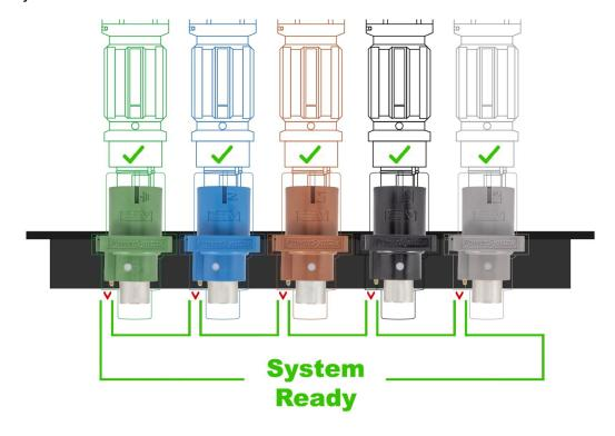
The connectors are keyed, polarized and color coded to prevent insertion of wrong phases.
